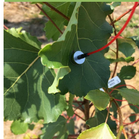
Using ZIM sensors to measure water potential in the field
